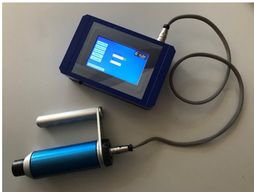
Figure 21. The commercial version of the B-RAD by ELSE NUCLEAR. The probe can also be mounted on an extension rod for measurements at a distance.
