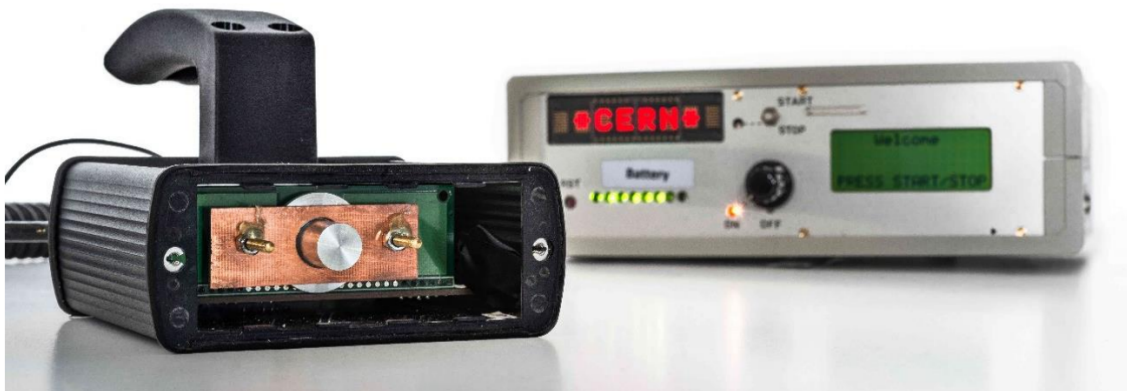
Figure 1. B-RAD. On the left, the probe with the front cover removed. The cylindrical case of the scintillating crystal is visible, sitting on the board housing the SiPM. On the right, the front panel of the control unit. The ON/OFF rotary switch, the Start/Stop button, the LED indicators for the battery status, the LED display (showing “CERN”) and the liquid crystal display can be seen.
