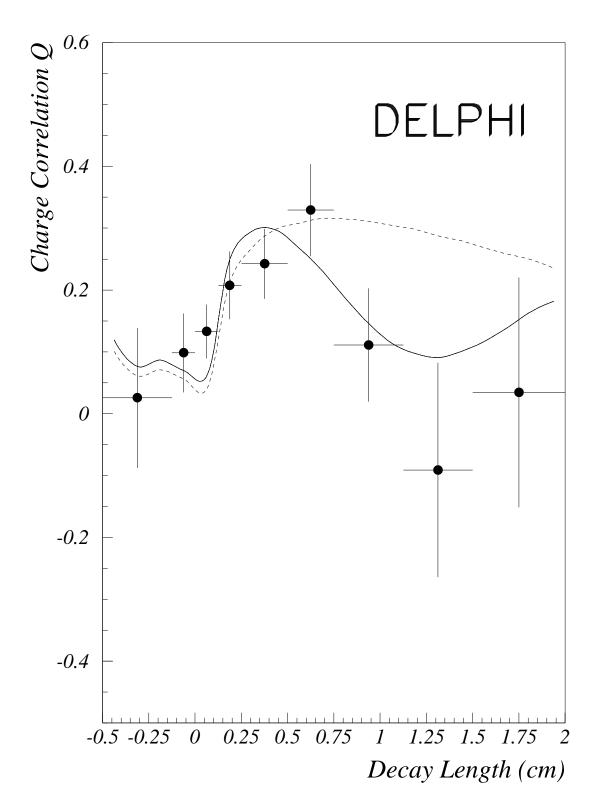
Figure 3: The charge correlation function Q plotted as a function of the  $D^0$  decay length in cm. The full dots with the error bars represent the data. The full curve is the result of the fit corresponding to  $\Delta m = 0.50 \ \hbar/ps$ . The dashed curve corresponds to a time independent mixing hypothesis.
