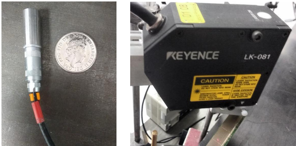
Figure 4: Displacement sensors. Capacitive sensor head (left), laser triangulation sensor (right). Note laser point on device under test at bottom.
