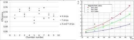
**Fig. 5.** Left: GEM chamber efficiencies measured in the deuteron beam run in December 2016. Right: The average trajectories of the deuteron beam and the average Lorentz shifts of an electron avalanche in 6 GEM planes measured for three values of the magnetic field.
