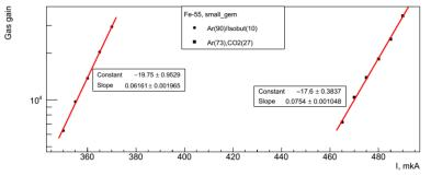
Fig. 3. The GEM gas gain for the  $Ar(70)/CO_2(30)$  and  $Ar(90)/C_4H_{10}(10)$  gas mixtures as a function of the current in the high voltage divider
