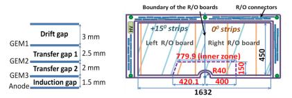
Fig. 2. Left: Schematic cross section of BM@N triple GEM detector. Right: Schematic view of the big GEM detector.
