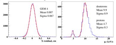
**Fig. 6.** Left: GEM hit residuals for experimental data. Magnetic field 0.79 T. Right: Momentum resolution for deuteron beam ~9%. Momentum resolution for proton spectators ~6%.
