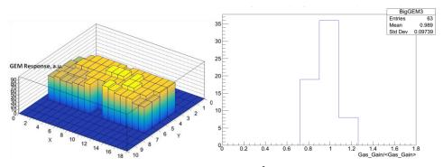
Fig. 4. Gas gain uniformity measurements for  $163 \times 45$  cm<sup>2</sup> GEM chamber. Left: Response uniformity 3D plot. Right: Gas gain distribution normalized on average gas gain.
