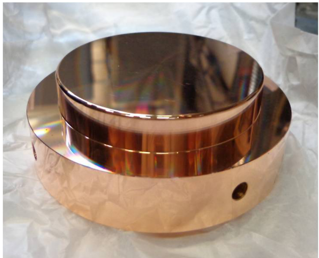
FIG. 1. An electrode used by the Large Electrode DC Spark System. The inter-electrode vacuum gap is formed between the top surface of the electrode, and the same surface on an identical top electrode facing it symmetrically. The outer rim of the electrode supports the ceramic spacer that holds the electrodes apart and determines the vacuum gap distance. Electrode edges are gently rounded (rounding radius \gg gap distance) to prevent breakdown through the ceramic, and to reduce field enhancement by the edges.
