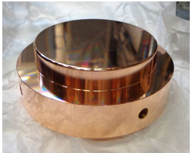
FIG. 1. An electrode used by the large electrode dc spark system. The interelectrode vacuum gap is formed between the top surface of the electrode and the same surface on an identical top electrode facing it symmetrically. The outer rim of the electrode supports the ceramic spacer that holds the electrodes apart and determines the vacuum gap distance. Electrode edges are gently rounded (rounding radius 1 mm) to prevent breakdown through the ceramic and to reduce field enhancement by the edges.
