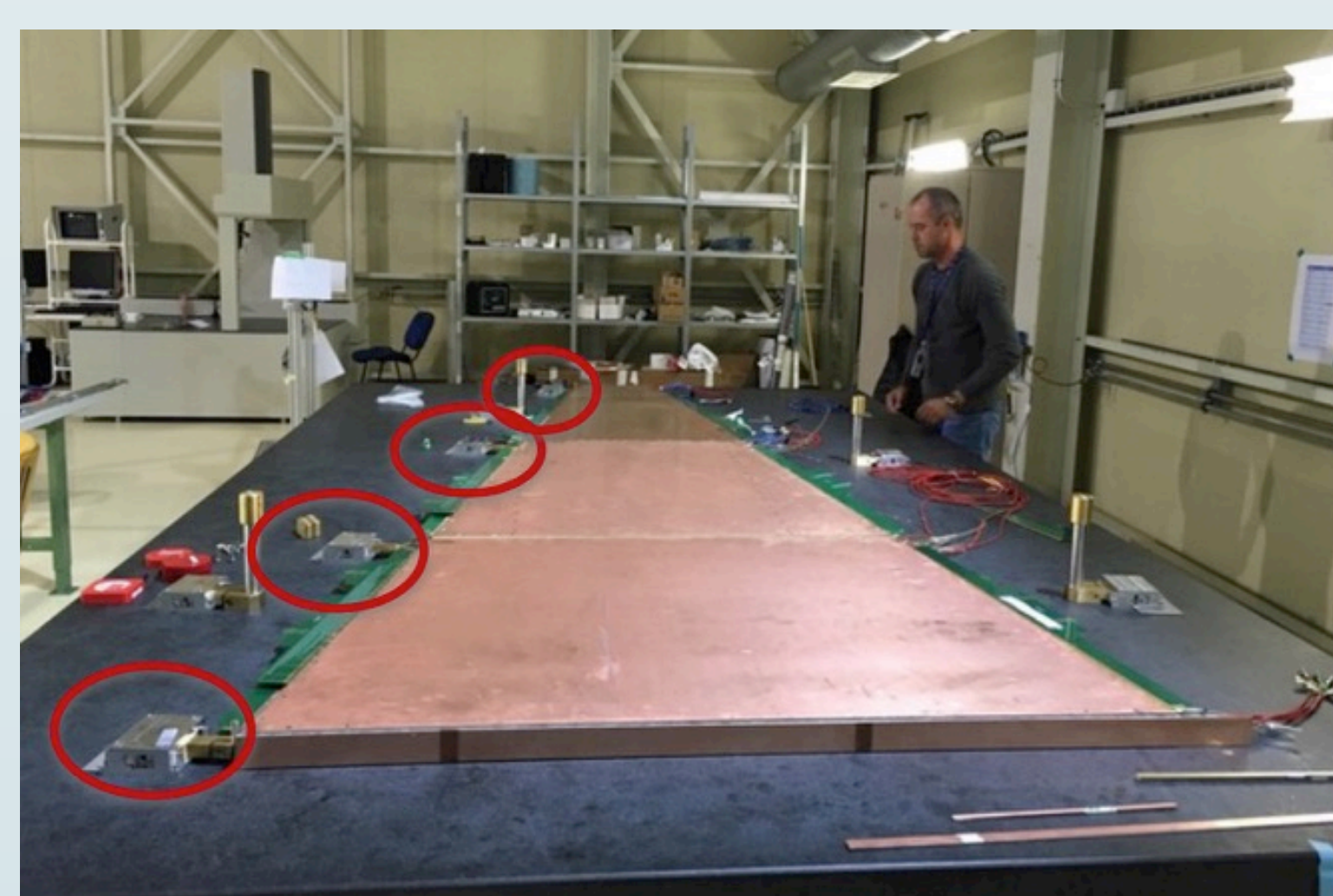
Figure 14: Wedge assembly. The brass features pushed against the alignment pins are marked in red circles
