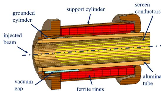
Figure 1: Details of the existing MKI beam screen.
