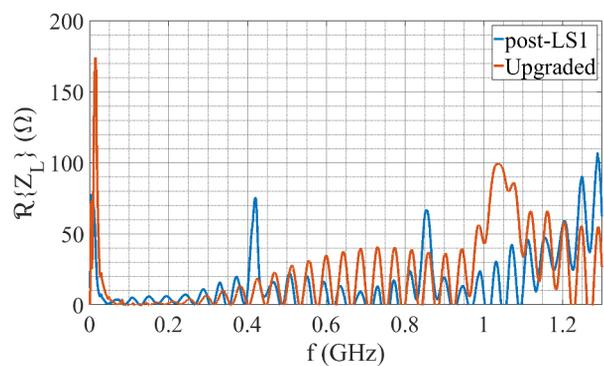
Figure 4: RLI measurements using the classical wire method.
