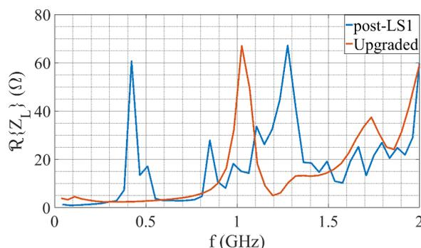
Figure 5: RLI measurements using the resonant method.
