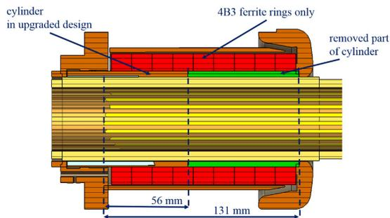
Figure 2: Changes in the upgraded MKI beam screen.
