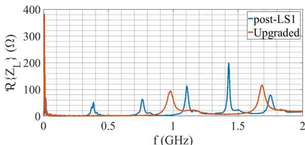
Figure 3: Predicted RLI for the post-LS1 and upgraded MKI beam screens.
