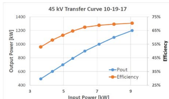
Figure 8: L3 MB-IOT: Output power and efficiency as a function of drive for 45 kV beam voltage with a 400 \mu\text{s} flat top and a 14 Hz repetition rate measured at CERN.
