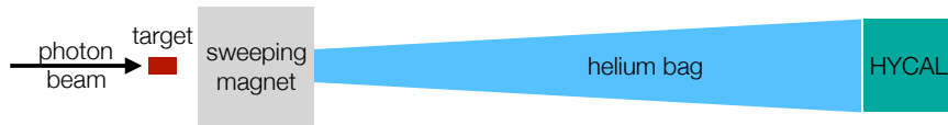
FIG. S1: Schematic of the PRIMEX experiment (not to scale) including the high-resolution multichannel calorimeter (HYCAL) which is vital to the search proposed here.
