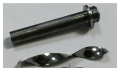
Fig. 5. Photograph of the transfer tube and associated helical chicane.
