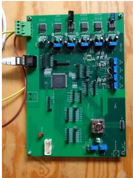
Figure 7: The test board for testing packaged chips
