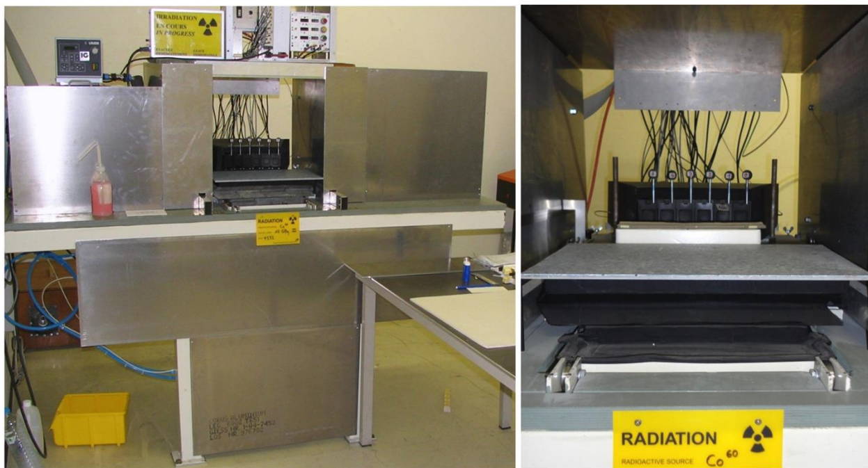
Fig.17: Pictures of the Co60 radioactive source used for studies on radiation hardness.
