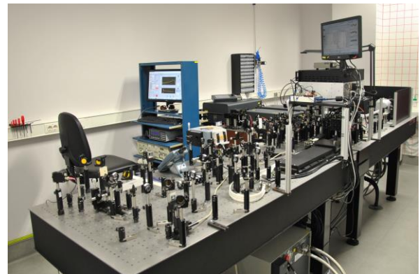
Fig. 9.: Schematic outline of pump and probe configurations Fig. 10: Test bench for pump and probe study
