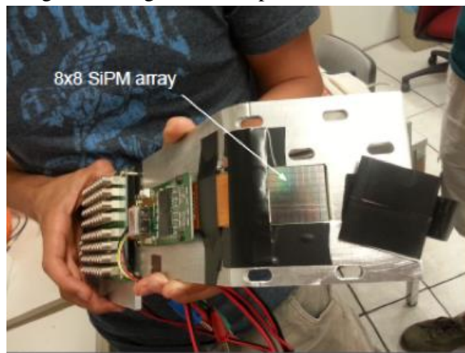
Fig. 30: SPACAL Setup showing the SiPM array
