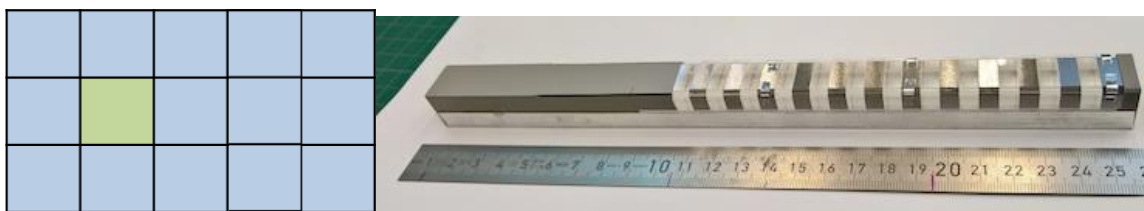
Fig. 21. Left: Layout of the \text{W-CeF}_3 matrix. Right: Photograph of one matrix channel during assembly.
