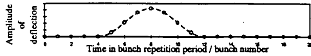
Figure 2-b Fast kicker deflection on the different bunches for 4 bunches in the rise time of the fast kicker
