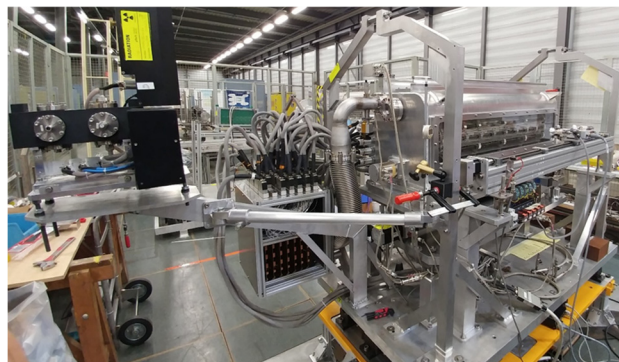
Figure 1: View of the Multimat test-bench. Beam comes from the left traversing embarked beam monitors (in black). The rotatable barrel is visible behind the camera window.
