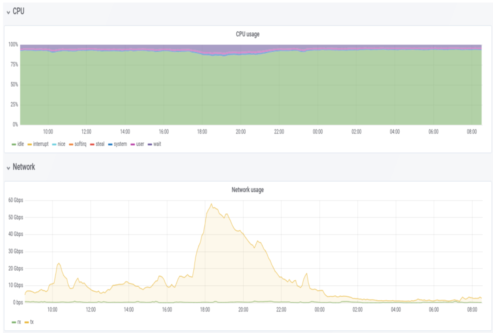
Figure 1. CPU load and network interface usage of storage servers in a CERN EOS cluster over a 24 hour period.
