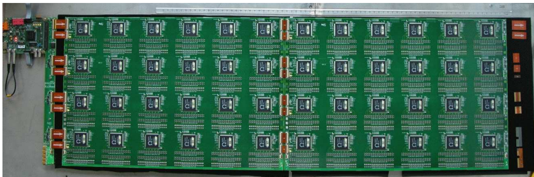
Figure 10. Photograph of two PCBs equipped with 24 HARDROCs each. The active area of a PCB is 32 \times 48 \text{ cm}^2 .
