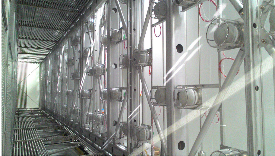
Figure 1. PMT deployment behind a TPC wire plane.
