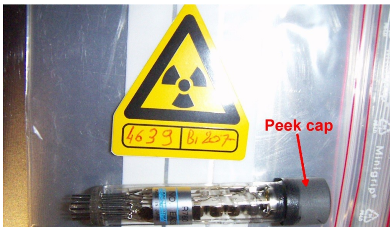
Figure 7. Photo of one of the Hamamatsu R760 photomultipliers with a ^{207}\text{Bi} source under the PEEK cap.
