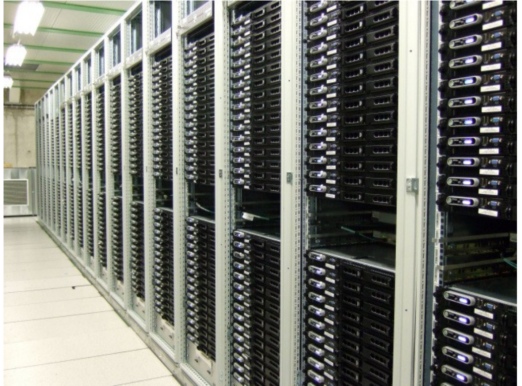
Processing farm for the ATLAS Data Acquisition System (DAQ), ~1900 machines, ~40k CPU cores (Picture from 2014)
