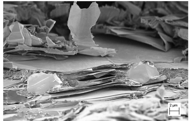
Fig. 9. SEM close-up of a fracture surface perpendicular to graphite basal planes. Grade MG-6541Aa. Image shows the edge of a graphite flake with two bonded carbide particles.
