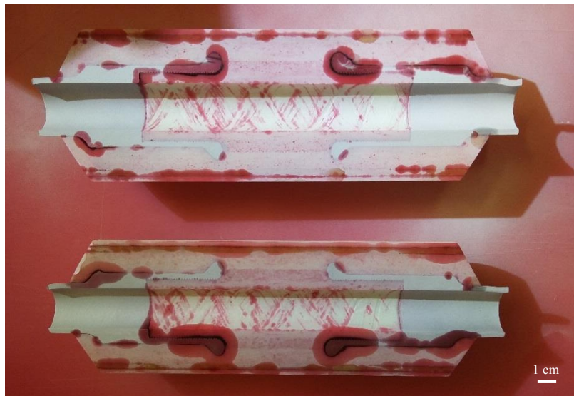
Figure 8. IBDH109 after application of developer. Dwell time: 20 minutes.
