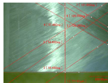
Figure 11. Fiber angle measurement for the inner composite of IBDH109.
