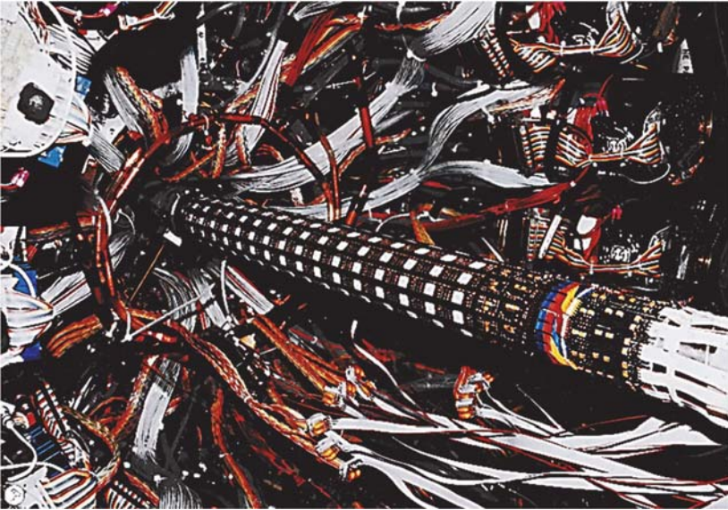
Fig. 6.17. Insertion of the inner silicon pad detector into the UA2 detector.
