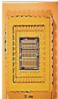
Fig. 6.15. ASIC AMPLEX, a 16 channel readout system developed for the Inner Silicon Pad Detector.
