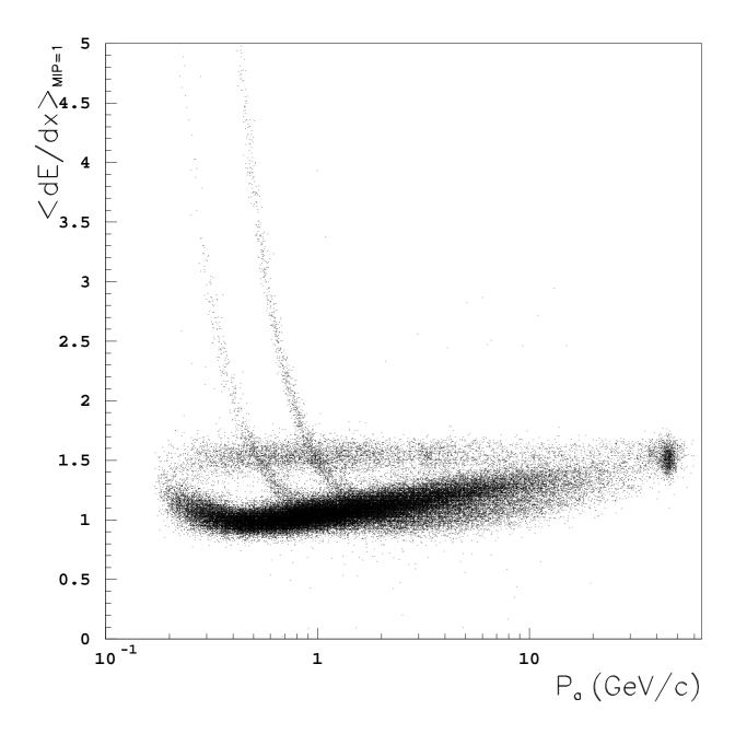
Figure 2: A scatter-plot of the truncated mean, normalized to unity for minimum ionizing particles, versus the apparent momentum is shown from a sample of events from 1989 and 1990 data which have been preselected for candidates. Only one in ten tracks outside the search regions is entered in the plot.
