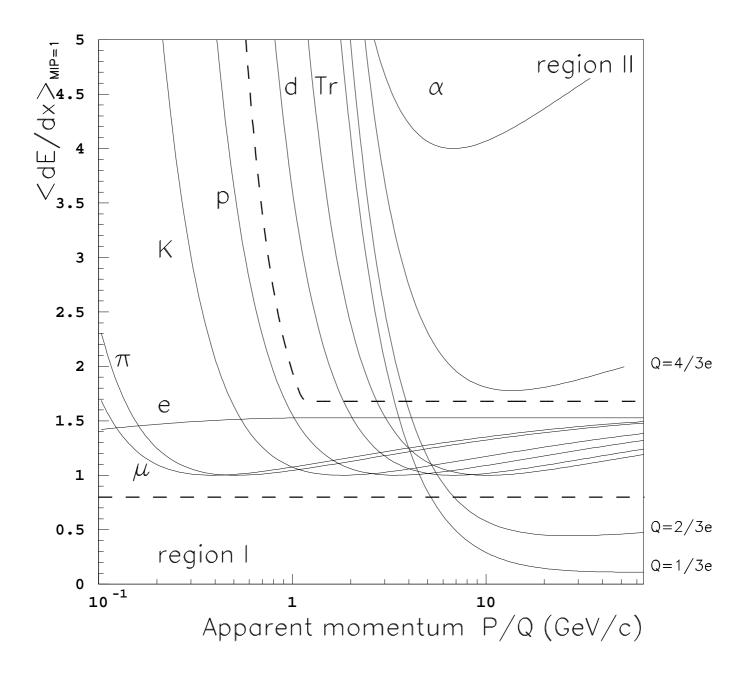
Figure 1: The expected ionization curves for different particle types. The curves for the fractional charges are for a mass  $5 \text{ GeV}/c^2$  particle. The boundaries for the search regions are displayed in the case of an average resolution.
