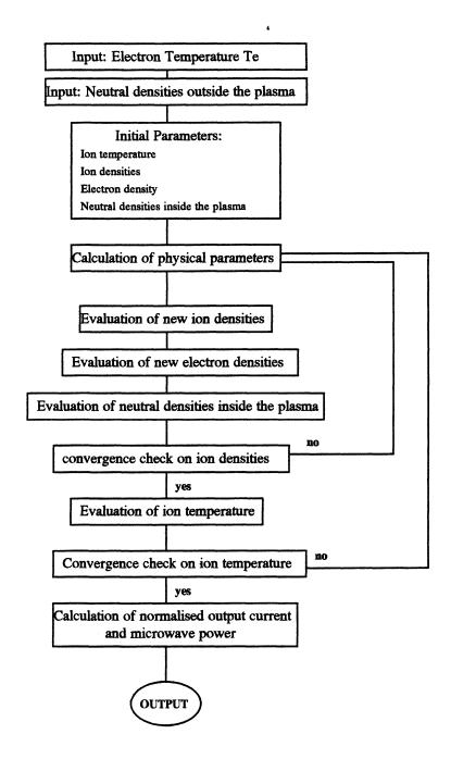
Fig.1 Schematic diagram of the computational method
