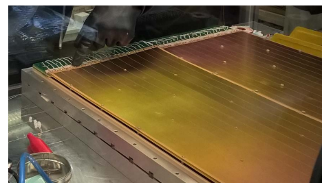
Figure 4: Picture, taken during the detector construction, of two THGEMs arranged in a detector. The 12 physical segments of each THGEM are visible.
