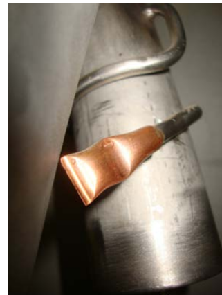
Figure 9: Cold welded filling tap.
