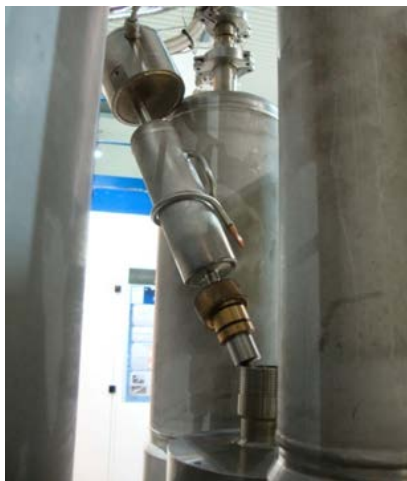
Figure 6: Pressure transmitter, ^3\text{He} tank with a filling pipe and capillary to ^3\text{He} bulb
