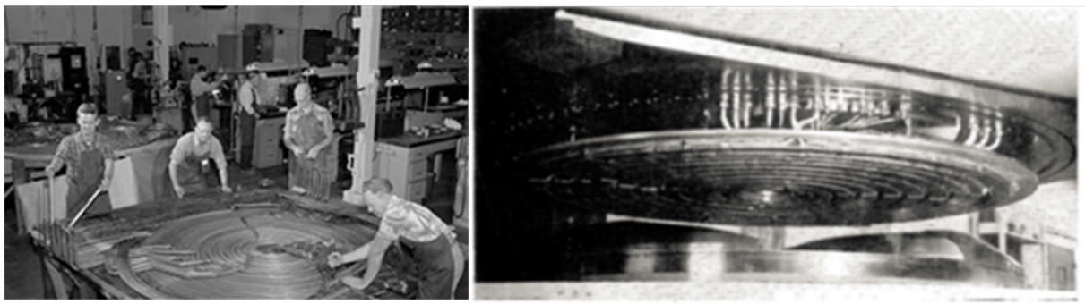
Fig. 24: A more general method is used to isochronize multiparticle variable-energy cyclotrons. Here, an array of concentric circular coils is placed on the pole and each coil uses its own independent power supply. In this way, there is a lot of flexibility in creating the required average magnetic field profile. Left: correction coils for the Berkeley 88-inch cyclotron [24]. Right: correction coils of the Philips 30 MeV azimuthally varying field cyclotron [23].
