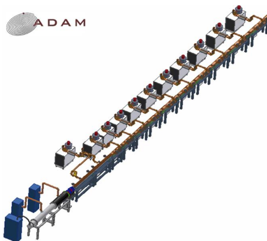
Fig. 17: Layout of a high-frequency linac for proton therapy, proposed by the CERN spin-off company A.D.A.M. (courtesy of A.D.A.M.).
