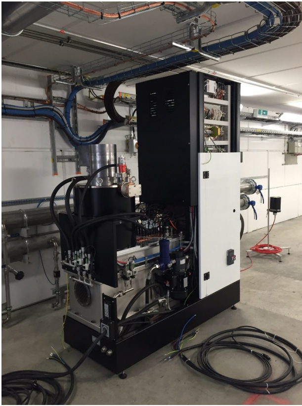
Figure 5: Modulator-klystron system installed at the ADAM test facility.
