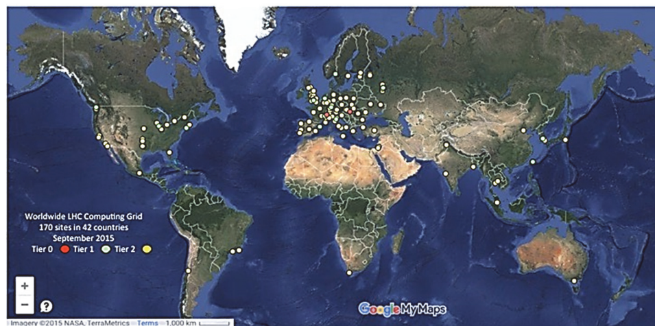
Fig. 9.4. A grid of 170 interconnected computing clusters in 42 different countries provide the processing capacity for analysing LHC data (Sept. 2015). Budapest and CERN are Tier 0 sites.
