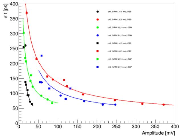
**Figure 2.** Time resolution achieved with the calorimeter cell using the signal of each of the SiPMs individually. The data for each SiPM consists of two sets, one with the DSB WLS plastic fiber and one with the capillaries with a liquid DSB based WLS. The time resolution improves with increasing signal amplitude. The best time resolution per fibre is around 60 ps for all of the channels. The amplitude at which this performance is achieved varies.
