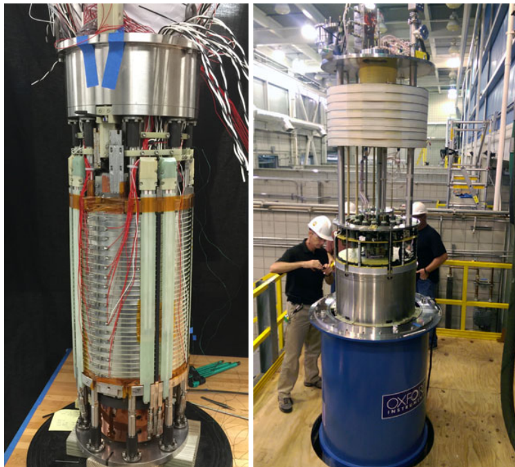
FIG. 23: Left: photograph of the innermost two high-Tc-superconductor (YBCO) coils of the all-superconducting 32 T magnet, whose successful operation was demonstrated in December 2017 at the NHMFL-Tallahassee. Total height of the pictured assembly is about 1 m. These YBCO coils are integrated within an outer coil set made of conventional (low-Tc) superconducting wire. The LTS outsert and the cryostat were designed and developed by Oxford Instruments NanoScience. Right: magnet assembly. Photos courtesy of the NHFML-Tallahassee.
