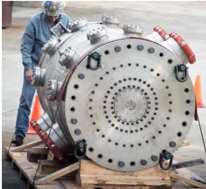
FIG. 20: Photograph of the 41.4T resistive magnet at the NHFML-Tallahassee (August 2017). This magnet has a 32 mm bore and is powered with a 32 MW power supply. Its design is based on Florida-Bitter plates (see text) using high-strength copper-silver-alloy conductor. Photo courtesy of the NHFML-Tallahassee.
