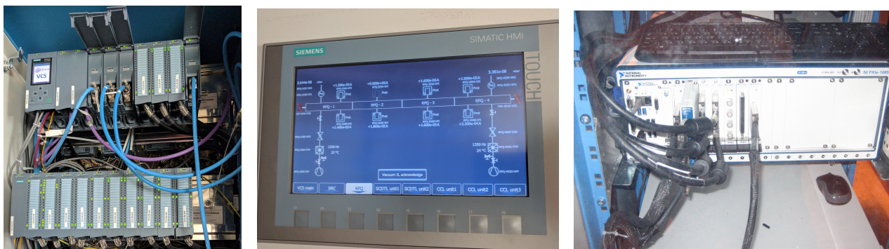
Figure 8: Vacuum Control (left), slow control touchscreen (middle) and beam diagnostics with BD Test Stand (right).
