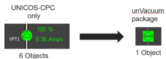
Figure 1: Turbomolecular pump widget without and with the vacuum package.
