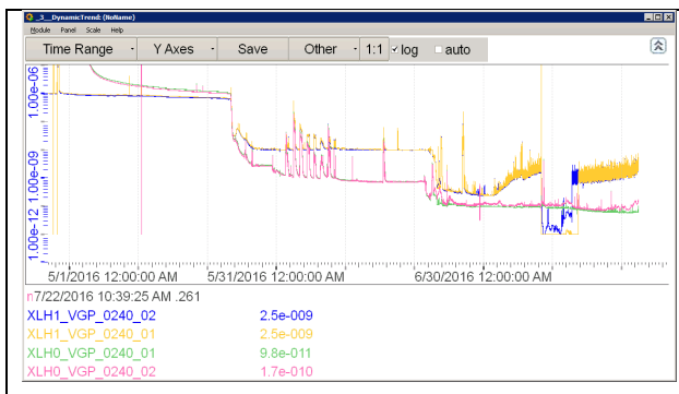
Figure 7: Vacuum pressure log of the two cryomodules.
