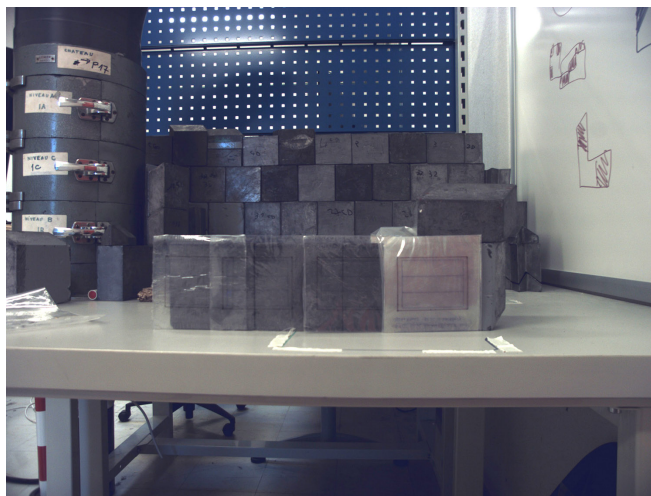
Figure 7. Combination of six planar ^{57}\text{Co} sources with 1716 kBq of total activity.
