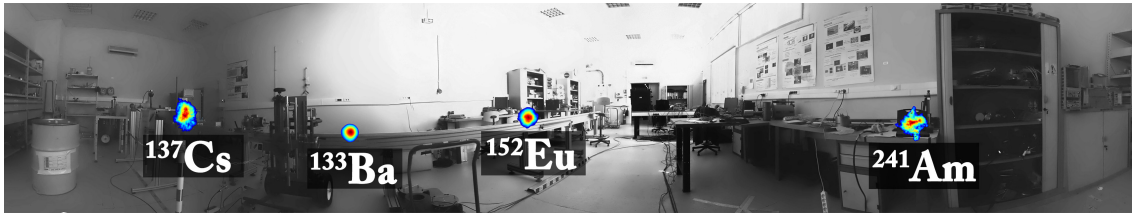
Figure 13. A panorama image with size 12574 \times 2316 pixels, with an horizontal and vertical FOV respectively of 360^\circ and 80^\circ , resulting from the stitching of 80 optical images and the superimposition of 4 \gamma -images. For illustration purposes, the image is shown in black and white.
