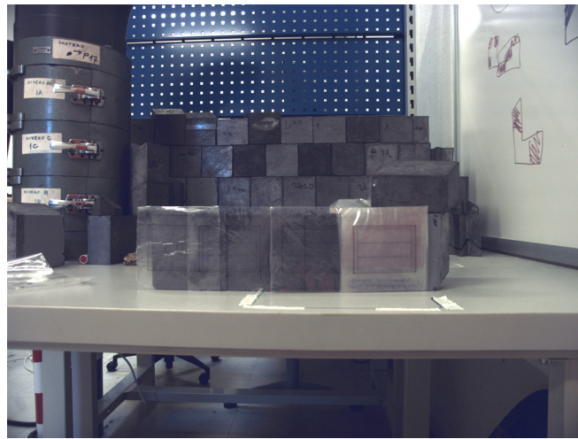
Figure 7. Combination of six planar ^{57}\text{Co} sources with 1716 kBq of total activity.
