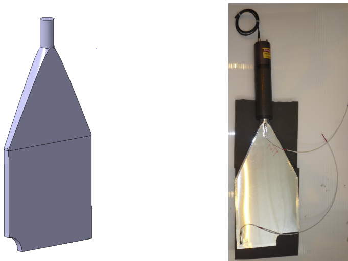
Figure 4. Schematic design of the scintillator and light guide of a single quadrant of B0/B1-type (47 mm inner radius), accompanied by a photograph of a B2/F2-type quadrant with the PMT and ‘clipping cable’ attached.
