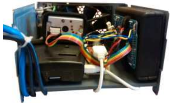
Figure 6. A DCES retro-fitted inside a standard ATX PSU: portable WIFI DCES.
