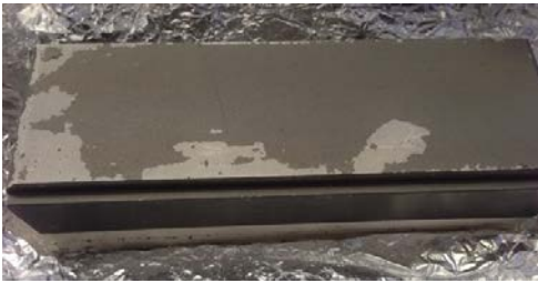
Figure 4: Coated boron nitride blocks after bake-out at 300^\circ\text{C} .
