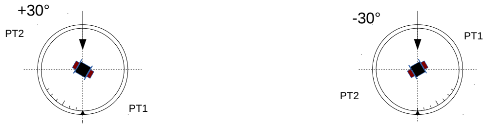
Figure 6. Setup of the test beam at BTF. The circular platform supporting the crystal could be rotated by \pm 30^\circ with respect to the incoming beam line (indicated by an arrow). Two detectors (PT1 and PT2) mounted on opposite sides of the scintillator collected the scintillation and the Cherenkov light.
