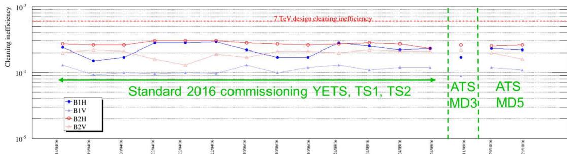
Figure 14: Summary of the betatron cleaning performance with 6.5 TeV beams during the Run II, in both planes of both beams. Cleaning measured during the proton-lead ion runs in 2016 are also reported.
