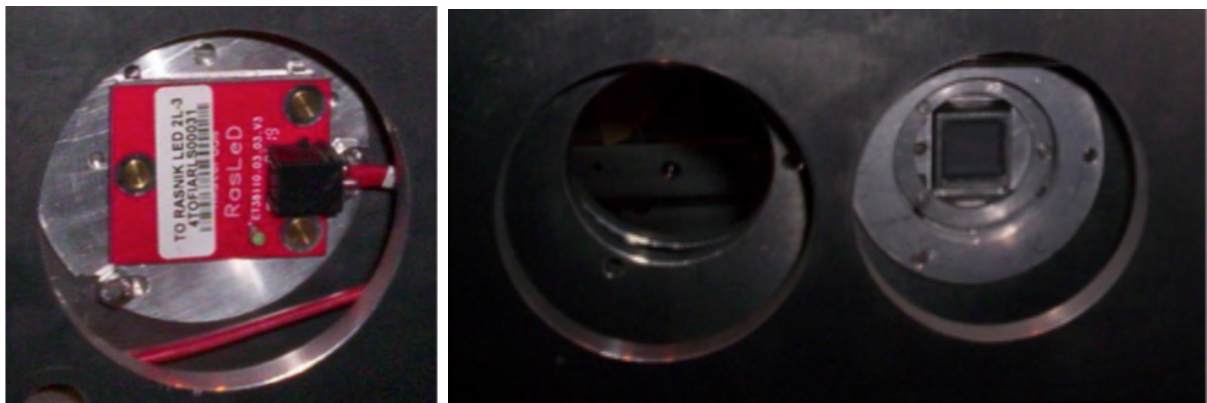
Figure 5: Two sides of a RASNIK mask mounted on a C-frame.
