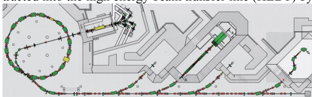
Figure 1: MedAustron accelerator layout: injector, synchrotron and extraction to four rooms including a Gantry.
