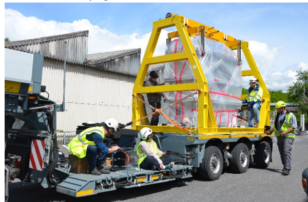
Figure 7: Transport of the first cryo module to the hall.
