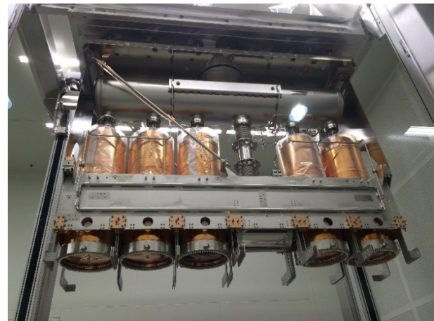
Figure 5: One of the final stages of CM1 assembly.
