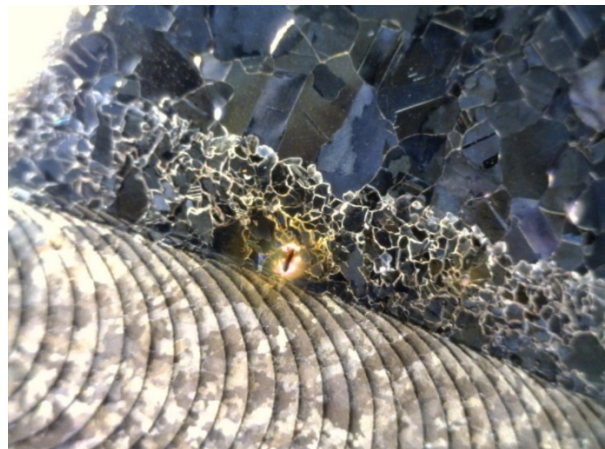
Figure 3: defect at the weld HAZ of the third cavity.
