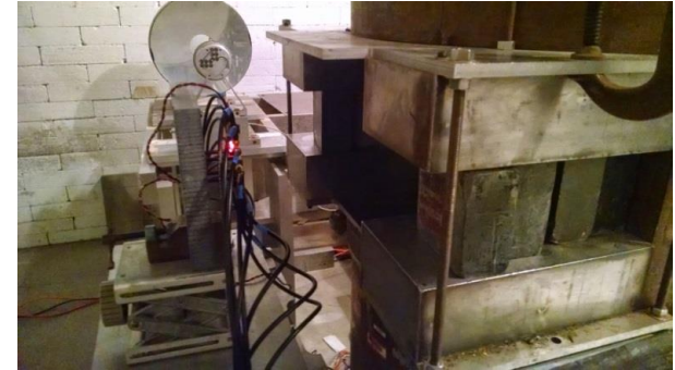
Repeater board @ Co-60 source location
