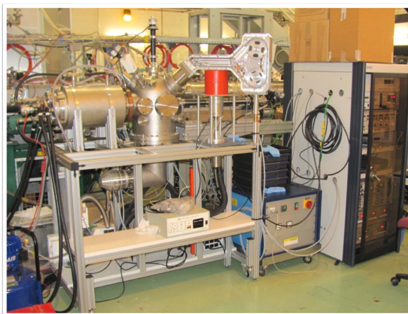
Figure 9. The newly commissioned online diffusion chamber which will allow diffusion studies of isotopes with half-lives in the minutes domain.
