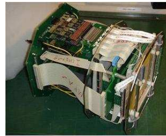
FIG. 3. (color online) Picture of SIMBA without its cylindrical coverage of 11.5 cm diameter.
