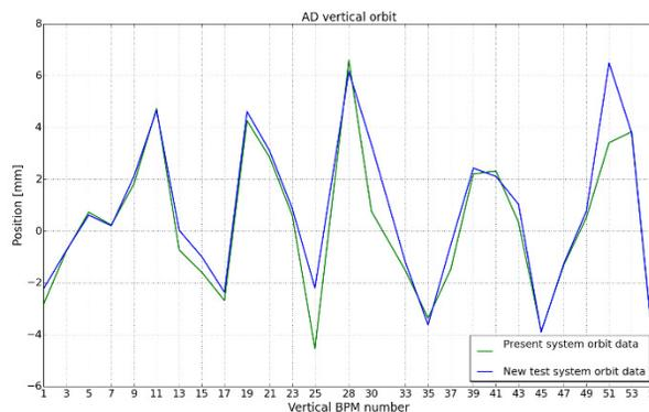
Figure 5: Position measurement all vertical BPMs acquired during the first AD flat top (at 35.77 s) with the current orbit system (green line) and the prototype version of new orbit system (blue line).
