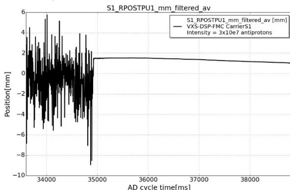
Figure 4: Position measurement for a vertical BPM acquired with the S1 VXS-DSP-FMC carrier during the first flat top and deceleration ramp in the AD cycle.
