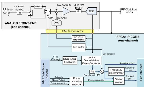
Figure 3: FMC-ADC board hardware and DDC firmware.
