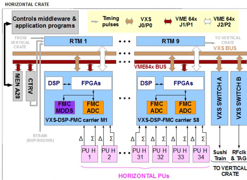
Figure 2: Digital acquisition system block diagram (horizontal crate). MDDS: Master DDS FMC board. ADC: Analogue-to-Digital FMC board. RTM: Rear Transition Module. CTRV: Timing Receiver Module. Men A20: master VME board. PU H: Horizontal transverse Pick-Up.
